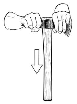
**Removal method #1:** Hold both sides of the head. With firm downward motions strike the handle end on something hard.
