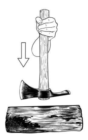
**Seating method:** Align the handle notch with the digging end of the head. Hold the handle firmly and strike downward onto something hard at least once.
