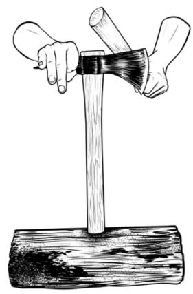
**Removal method #2:** Place the end of the handle on something hard. Hold one side of the head and strike the other side with a wooden baton. Alternate sides as needed.
